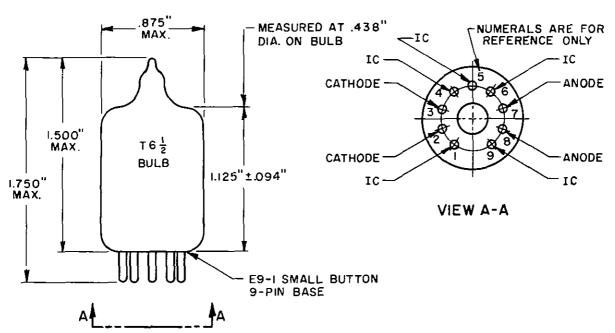
NOTE: PINS MARKED IC (INTERNAL CONNECTION) SHOULD NOT BE CONNECTED TO ANY PORTION OF AN EXTERNAL CIRCUIT. FAILURE TO OBSERVE THIS PRECAUTION MAY RESULT IN IMPROPER OPERATION OF THE TUBE.
